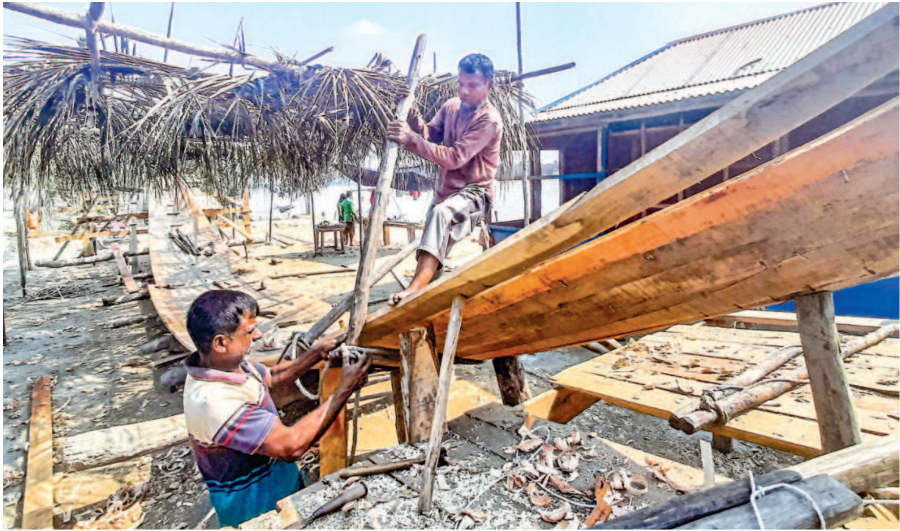
Carpenters are seen making a boat for fishing in the sea. Generally, they use the timbers of mahogany trees to build such vessels, which are normally 60 feet long and 12 feet wide. Around a month is needed to make such a boat at a cost of about Tk 6 lakh. The picture was taken at an area housing a community of fishermen called Sharafpur in Dumuria upazila of Khulna on February 12.
