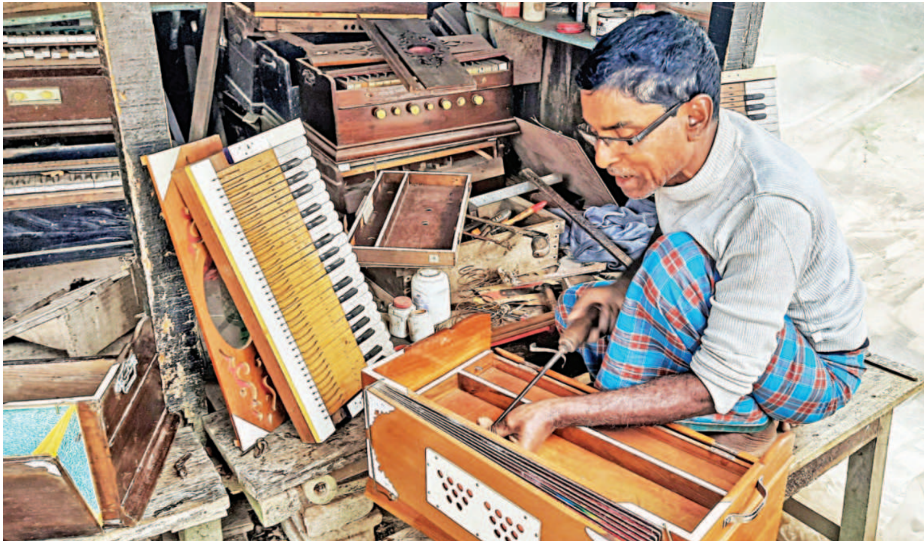
Nikhil Biswas has been making harmoniums for the past 18 years. The keyboard musical instrument works by wind being supplied by bellows. Making one takes him around 20 days and he can sell it for up to Tk 30,000. The photo was taken at Ruprampur village of Khulna's Dumuria upazila earlier this month. PHOTO: HABIBUR RAHMAN
