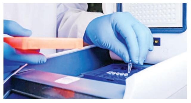
Polymerase chain reaction (PCR) machines are cost-effective and highly efficient tools used to amplify small segments of DNA or RNA that are selected from the genome using a primer.
