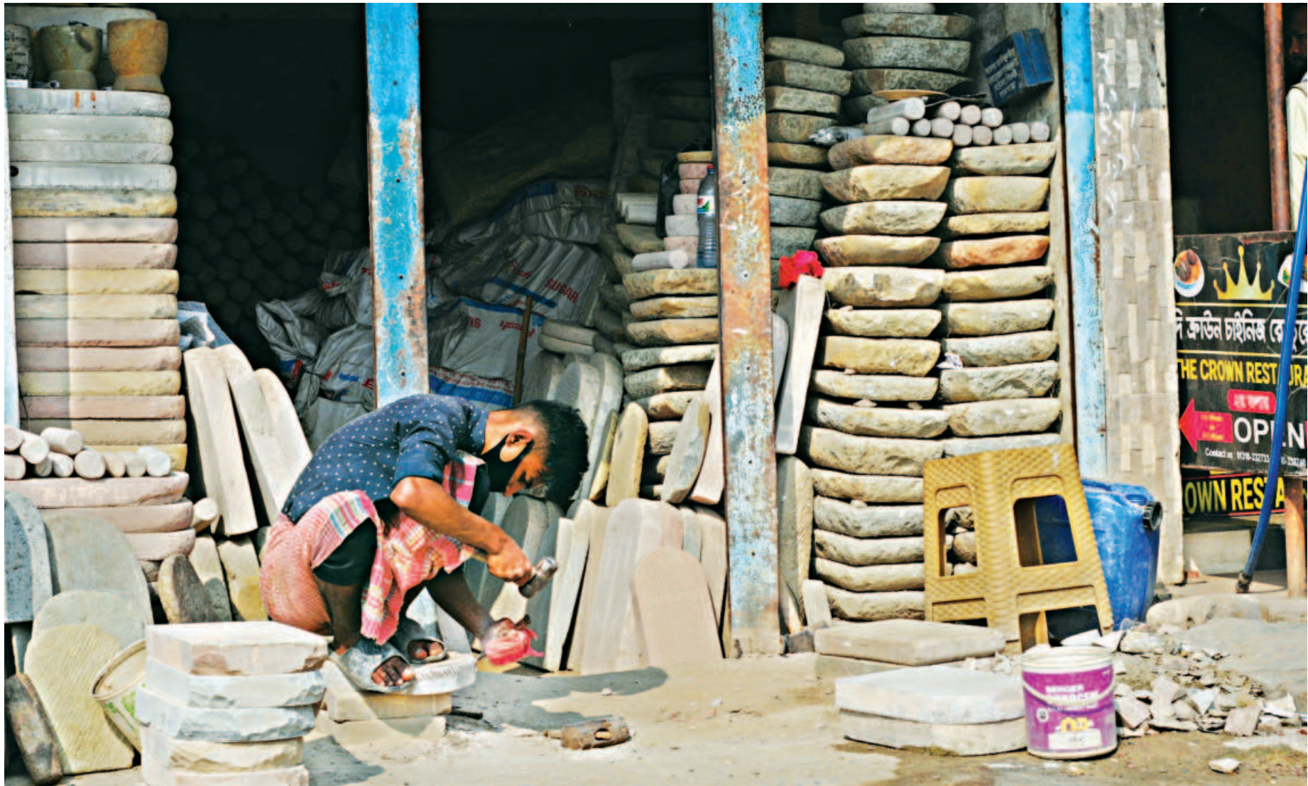
A craftsman uses a hammer and chisel to make a traditional grinding stone. The use of such grinding stones is on the wane for the advent of readymade masalas and mixes alongside modern and time saving gadgets. A set of grinding stones made from igneous rock sells for Tk 1,200 to Tk 2,500 while ones made from stone meant for construction for Tk 800 to Tk 1,500. The photo was taken in front of Sarada Hall in Sylhet city last week.
