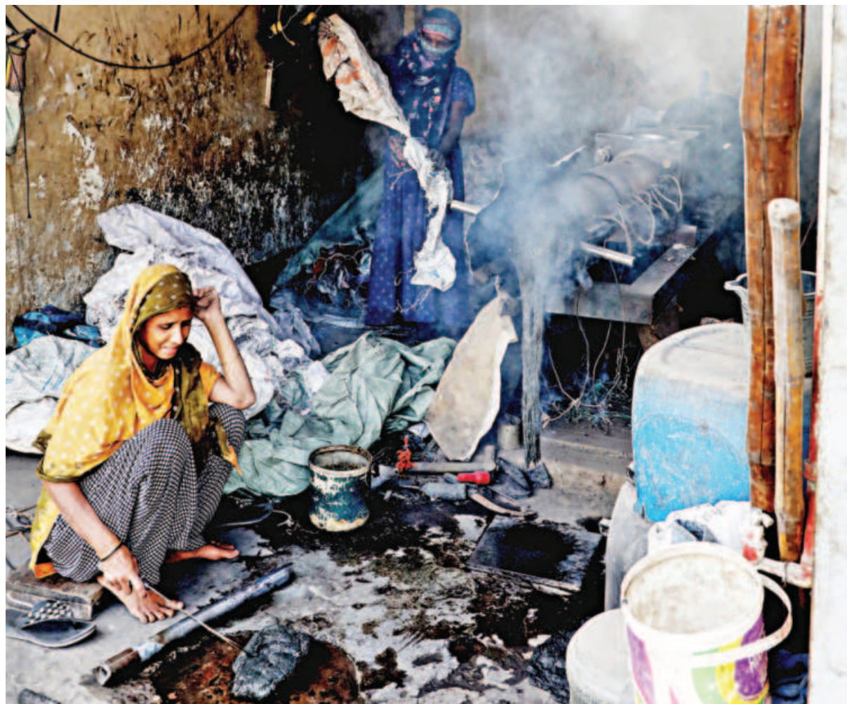
Workers in a plastic-scrap recycling workshop melt down the collected materials to turn them into solid blocks of plastic to be sold to recycling factories. They work amid severe health risks, as they have no protection to prevent the fumes from entering their lungs. In addition to that, these workshops inadvertently contribute to air pollution as they have no mechanism to filter out the toxic fumes. This photo was taken in Dhaka's Kamrangirchar recently.
