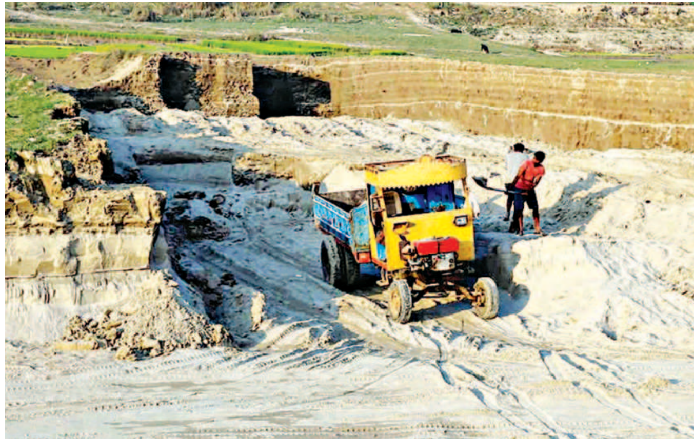
Sand being illegally hauled off the bed of the Padma in an area at the border of Pabna and Kushtia districts. The land will be under water during monsoon a few months later and the patch of depression on the river bed will disrupt the water flow, worsening erosion of the banks and putting nearby villages at risk. However, the ubiquity of such sand extractors in the two districts is a sign that the authorities are turning a blind eye to this.
