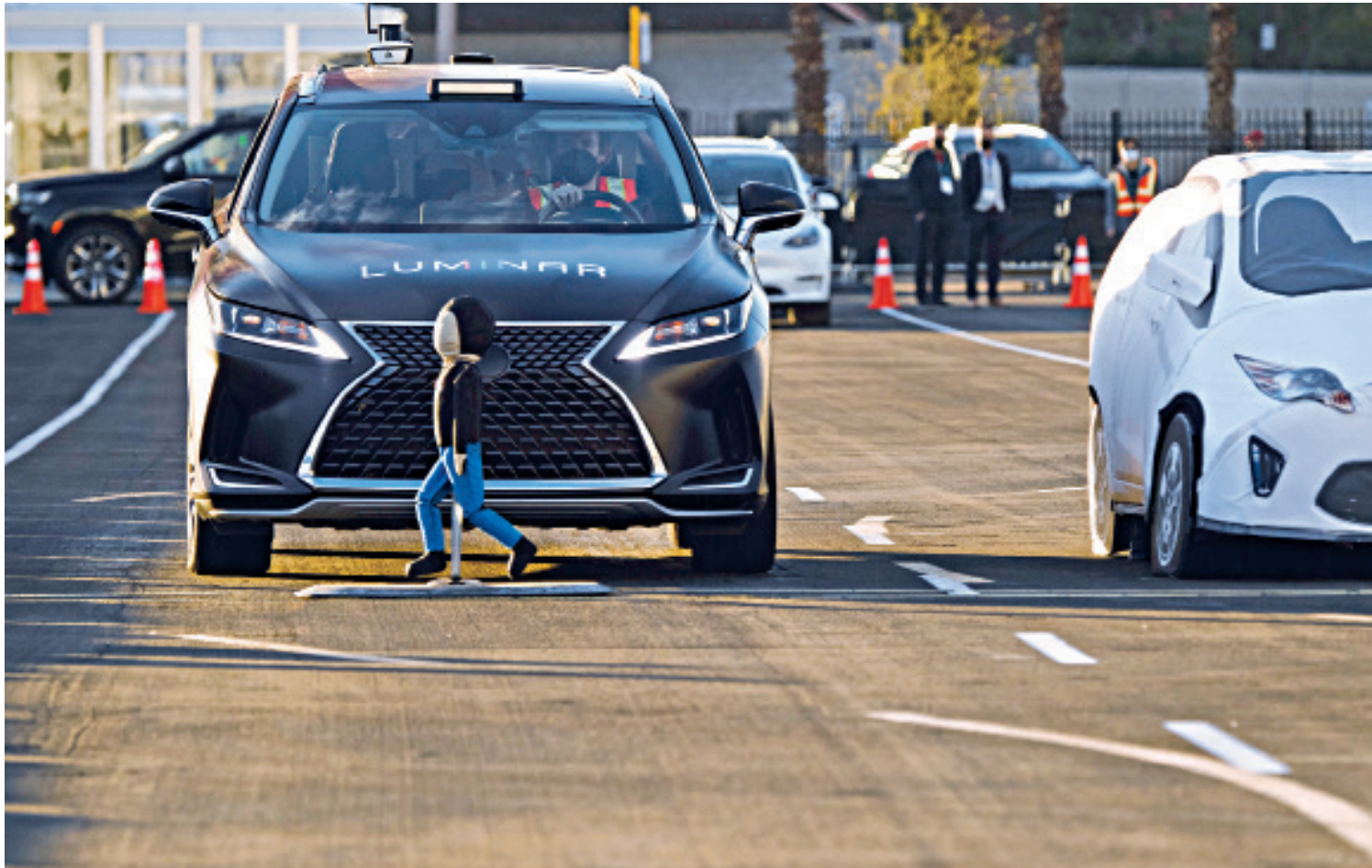
A vehicle with Luminar LiDAR based proactive safety pre-collision braking crash avoidance technology stops to avoid a child-sized test dummy as it is demonstrated on a test track at the Las Vegas Convention Center ahead of the Consumer Electronics Show (CES) on January 4 in Las Vegas, Nevada.
