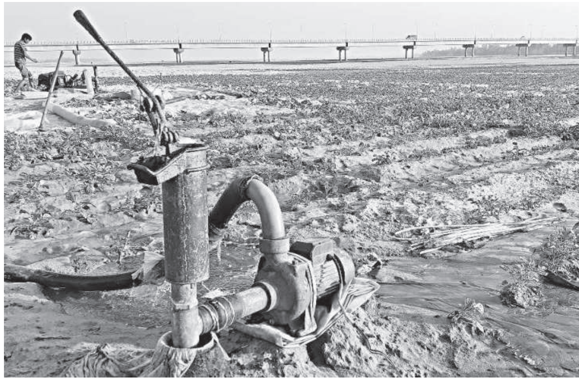
Farmers installed a diesel-run shallow machine in the dried-up Teesta riverbed to irrigate their crop field at Char Gokunda village in Lalmonirhat Sadar upazila.
