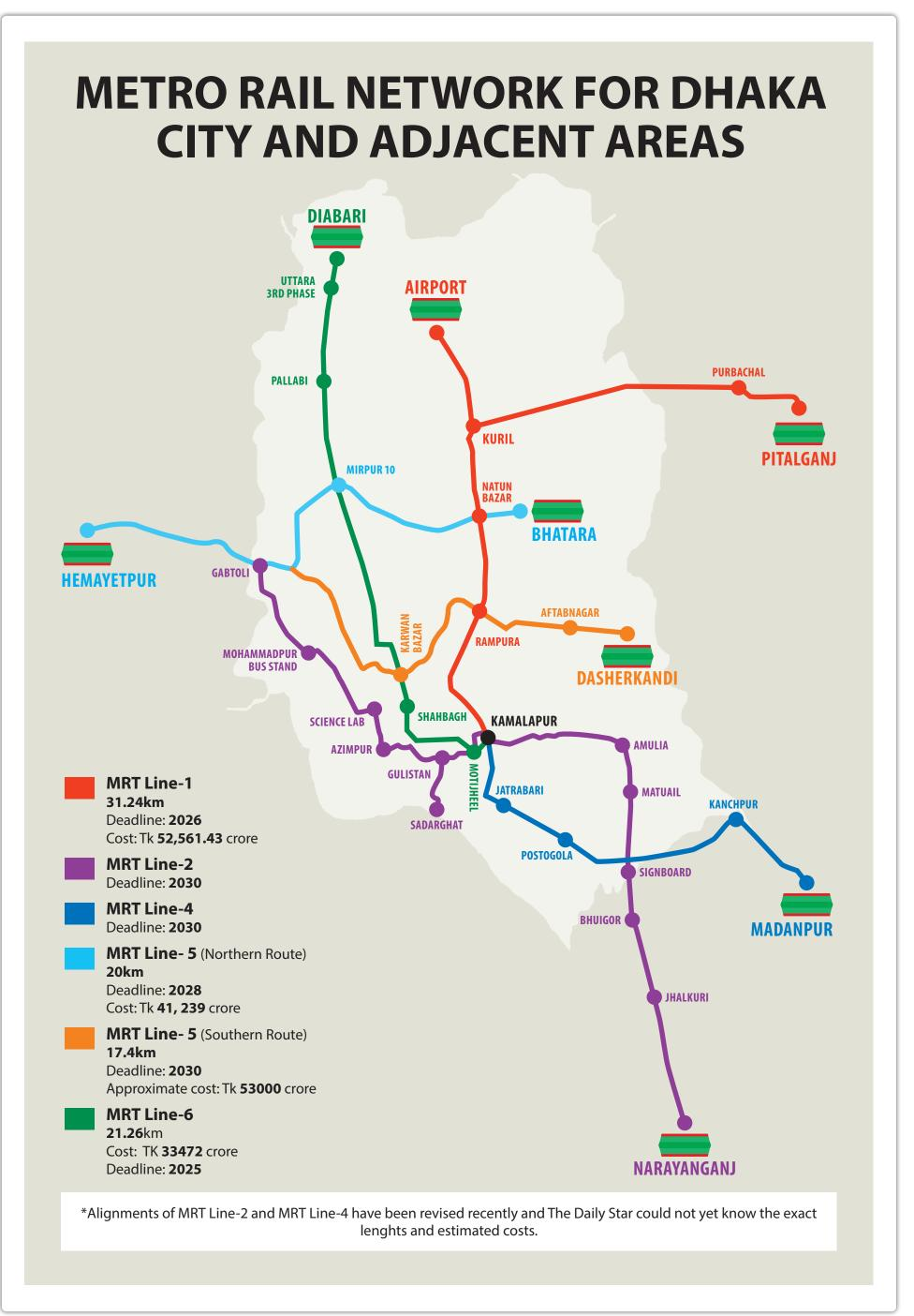
The 31.24km MRT Line-1 will have two parts: a 19.87km part from Hazrat Shahjalal International Airport, Khilkhet, Badda, Rampura, and Malibagh to Kamalapur (Airport route) which will be underground and an around 11.36km elevated line from Notunbazar to Purbachal (Purbachal route). The construction work of the Tk 52,561.43 crore project, the biggest infrastructure project in the transport sector and the first underground metro, is expected to start by February next year.
