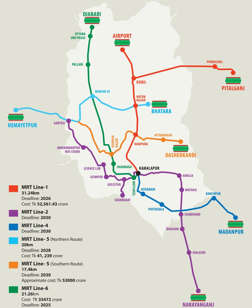
The 31.24km MRT Line-1 will have two parts: a 19.87km part from Hazrat Shahjalal International Airport, Khilkhet, Badda, Rampura, and Malibagh to Kamalapur (Airport route) which will be underground and an around 11.36km elevated line from Notunbazar to Purbachal (Purbachal route). The construction work of the Tk 52,561.43 crore project, the biggest infrastructure project in the transport sector and the first underground metro, is expected to start by February next year.
