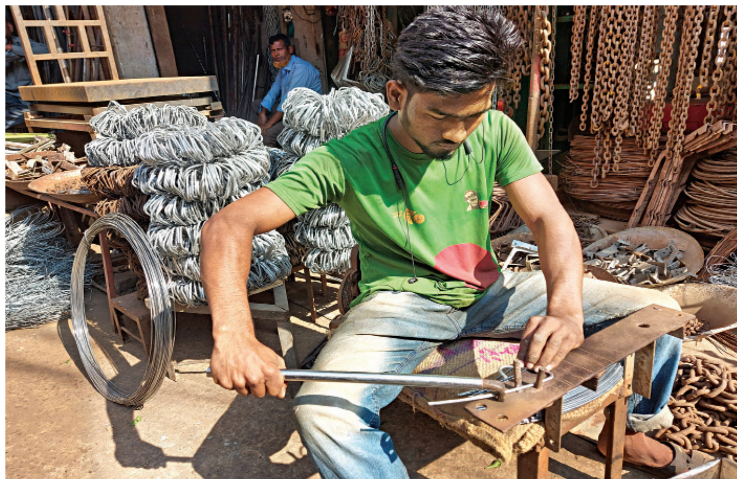
A worker creates closed loops of metal used in construction to strengthen rebars in beams and columns. Working from 9:00am to 8:00pm earns him Tk 300 a day. The photo was taken at Hatkhola area in Barishal recently.
