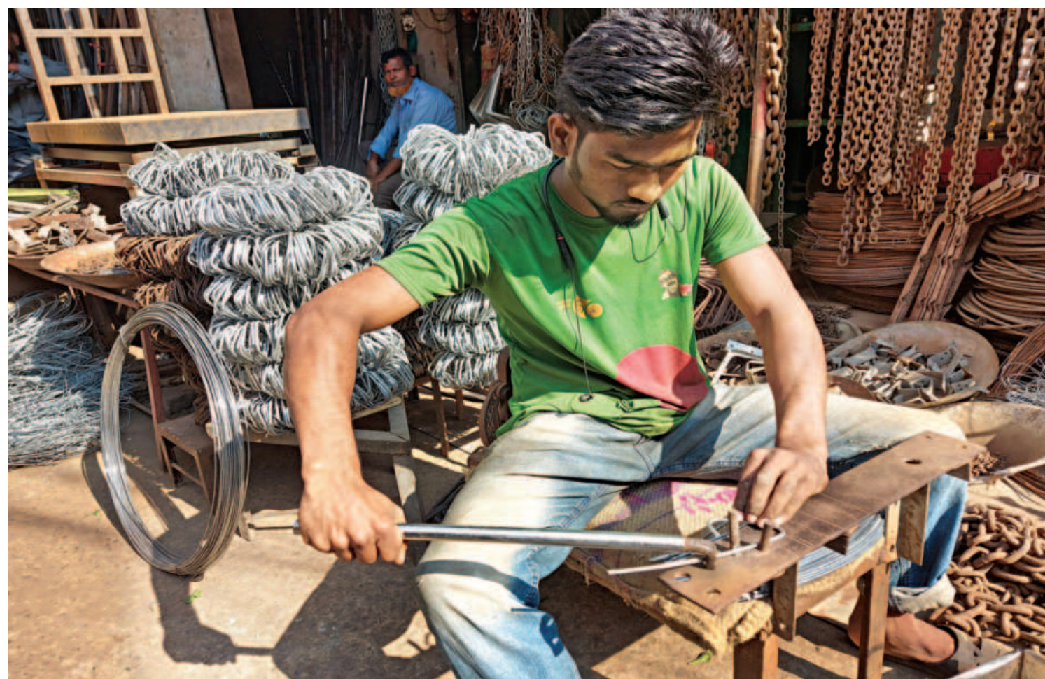
A worker creates closed loops of metal used in construction to strengthen rebars in beams and columns. Working from 9:00am to 8:00pm earns him Tk 300 a day. The photo was taken at Hatkhola area in Barishal recently. PHOTO: TITU DAS
