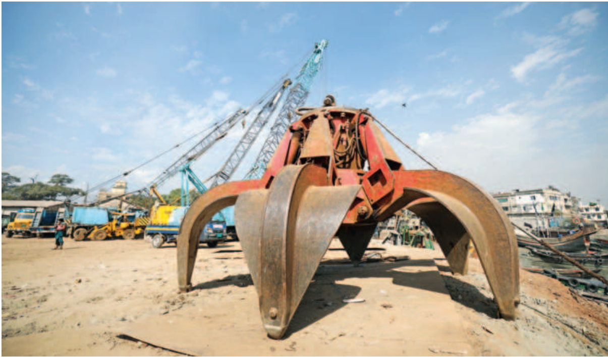
A detachable claw grabber, primarily used through cranes for unloading goods such as large stones and scrap metal from vessels, left idle at Anu Majhir Ghat in Chattogram city amidst a strike enforced by water transport workers since the early hours of yesterday demanding a pay hike.
