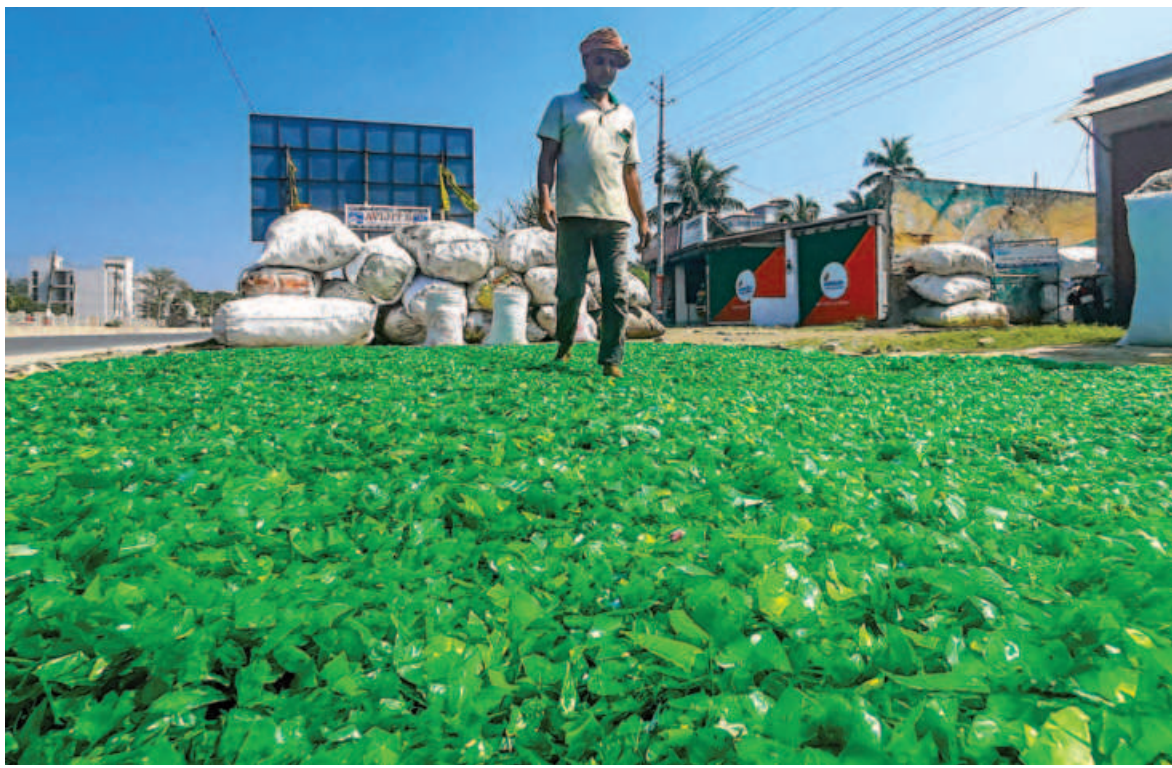
A worker dries pieces of plastic, which were procured after breaking down different bottles with a machine, under the sun. These scraps of plastic are then sold by the kilo to different factories that recycle and turn them into everyday-use items. This photo was taken in Khulna city's Zero Point area recently. PHOTO: HABIBUR RAHMAN
