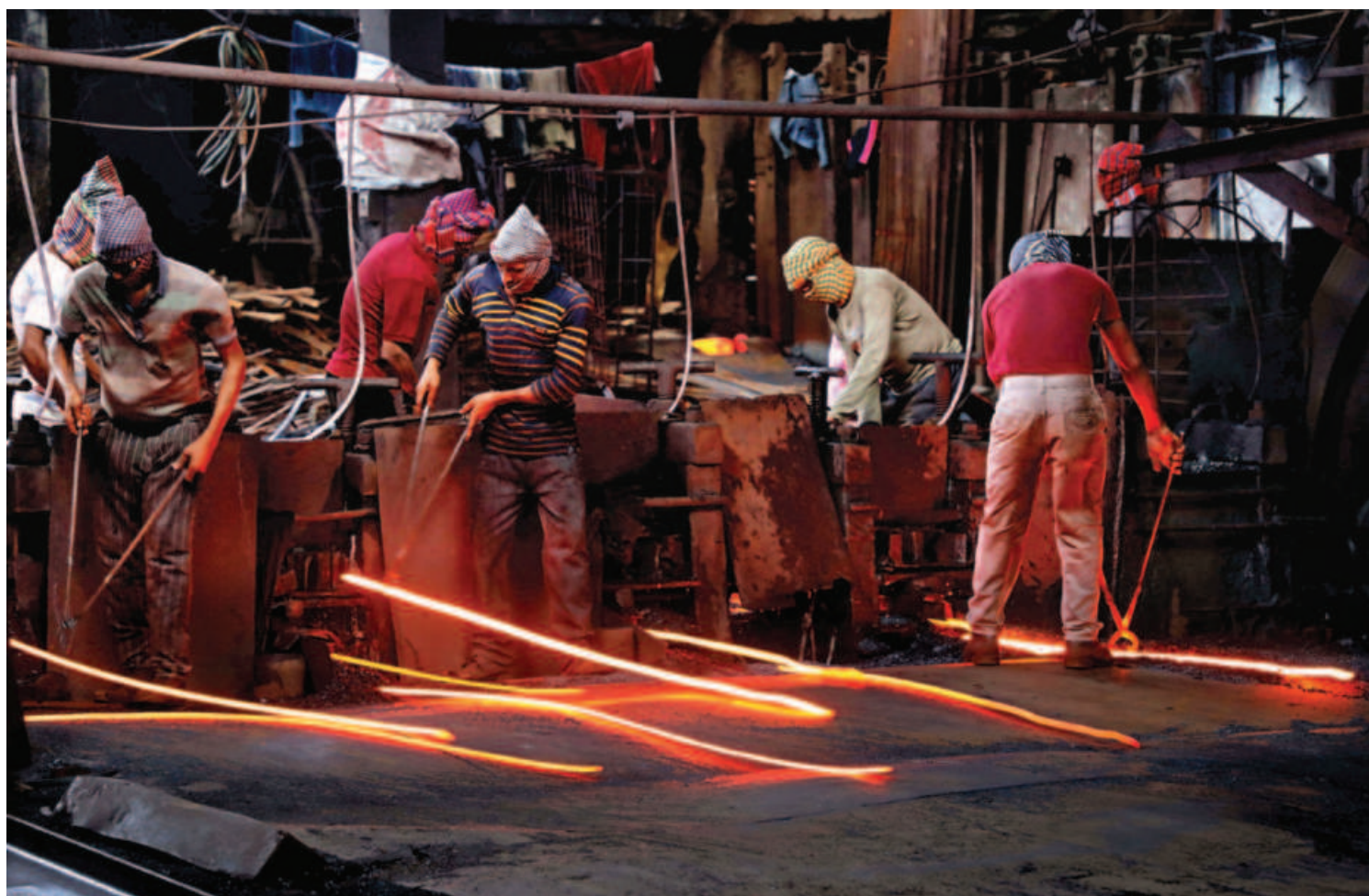
Working with molten metal involves multiple hazards. Besides the obvious risks of injuries caused by slips and trips at the foundry, the work entails chances of heat stress, heat stroke, and respiratory effects from exposure to the fumes to name a few. The photo of the men without proper personal protective equipment was taken at a re-rolling mill in the capital's Shyampur last week.
