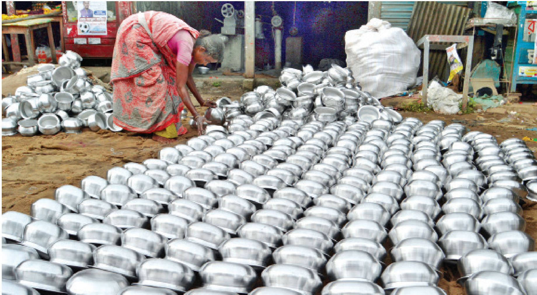
A worker sets aluminium cooking pots out in the open to dry after they have been washed on Bongobir Road in Sylhet city. The manufacturing process involves rotating a sheet of the metal at high speed on a spinning lathe and pressing a roller tool against it to achieve the desired shape. The price of aluminium kitchenware has increased by about 10 per cent to 20 per cent from Tk 350 per kilogramme in September last year, with industry insiders reasoning it to rising costs of business. The photo was taken last week.
