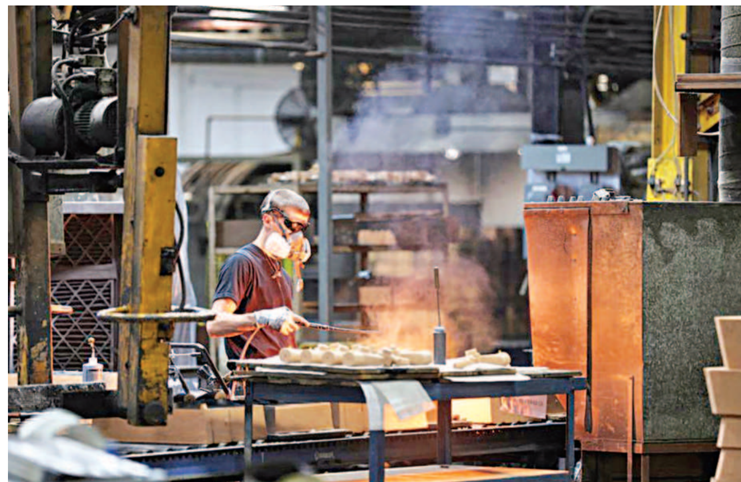
A worker does surface preparation of molds at Mitchell Aerospace, a manufacturer of light alloy sand castings for the aerospace industry, in Quebec, Canada on September 9.
