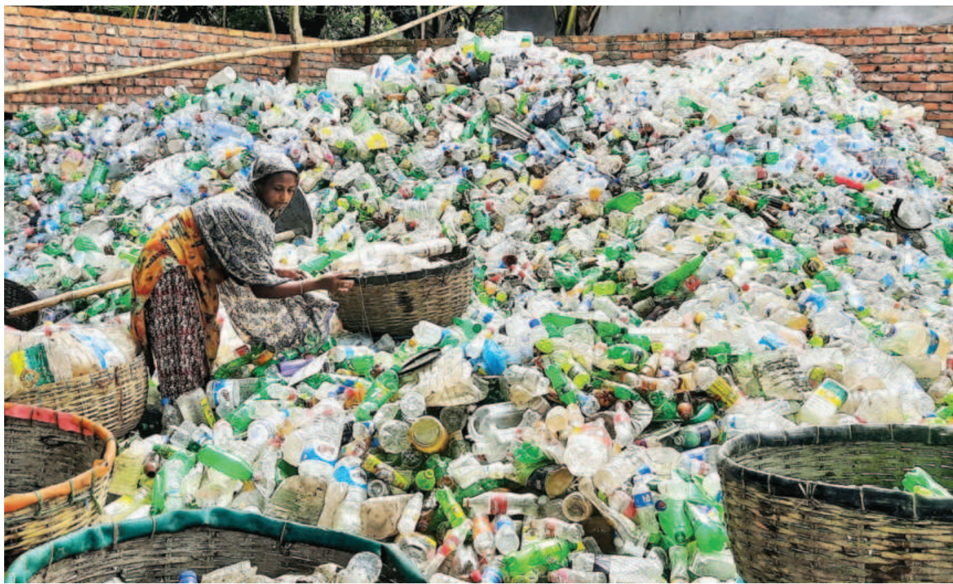
A worker sorts used plastic bottles by colour at a recycling factory in Khulna city's Khalishpur check post area yesterday. The labourer removes the caps and labels from the bottles before packing those in large bags. She can pack three bags a day and earns Tk 60 for each bag containing around 30-35 kg of plastic bottles.
