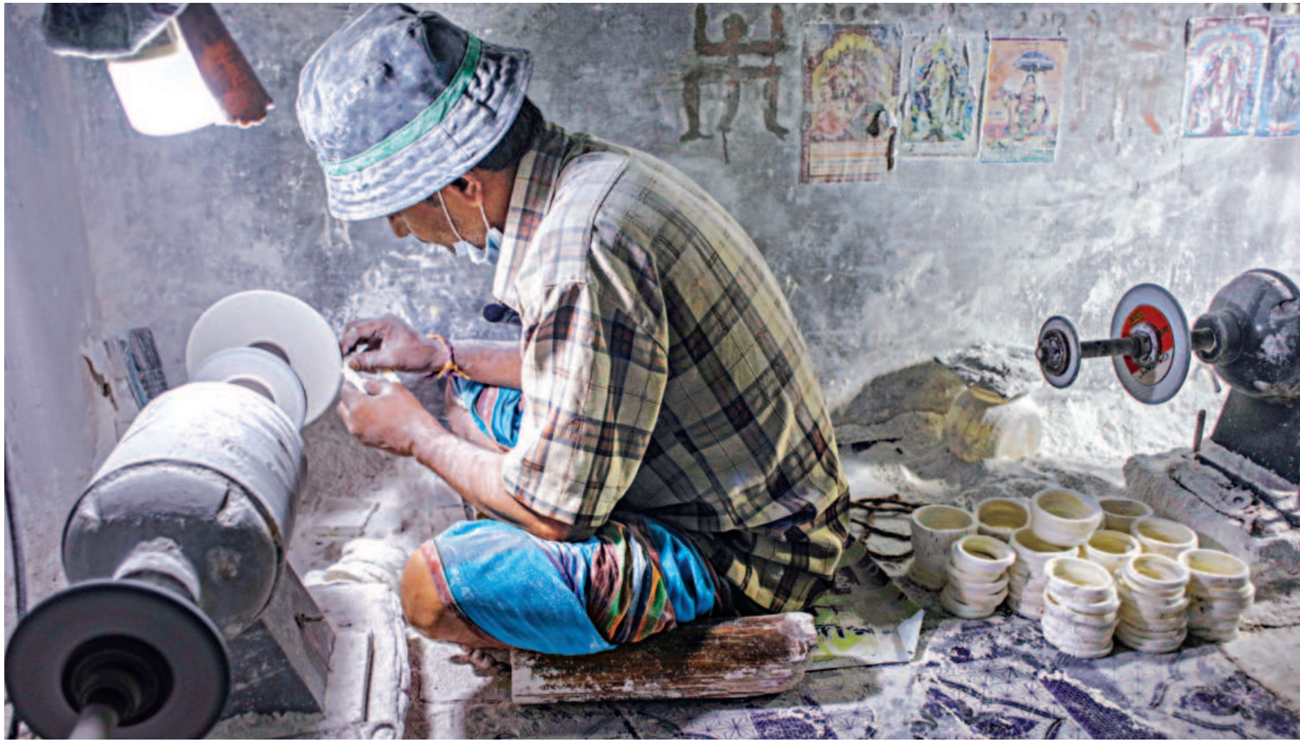
An artisan creates shankhas or white bangles made of conch shells at Shankhari Bazar in Dhaka. The centuries-old profession earns him Tk 25 per pair of bangles, traditionally worn by married Hindu women seeking well-being of their husbands. Designers used to cut conch shells by hand until machines were introduced a couple of decades ago. The shells are imported from Sri Lanka and India and each pair of bangles can sell anywhere from Tk 350 to Tk 6,000 depending on the designs. The photo was taken recently.
