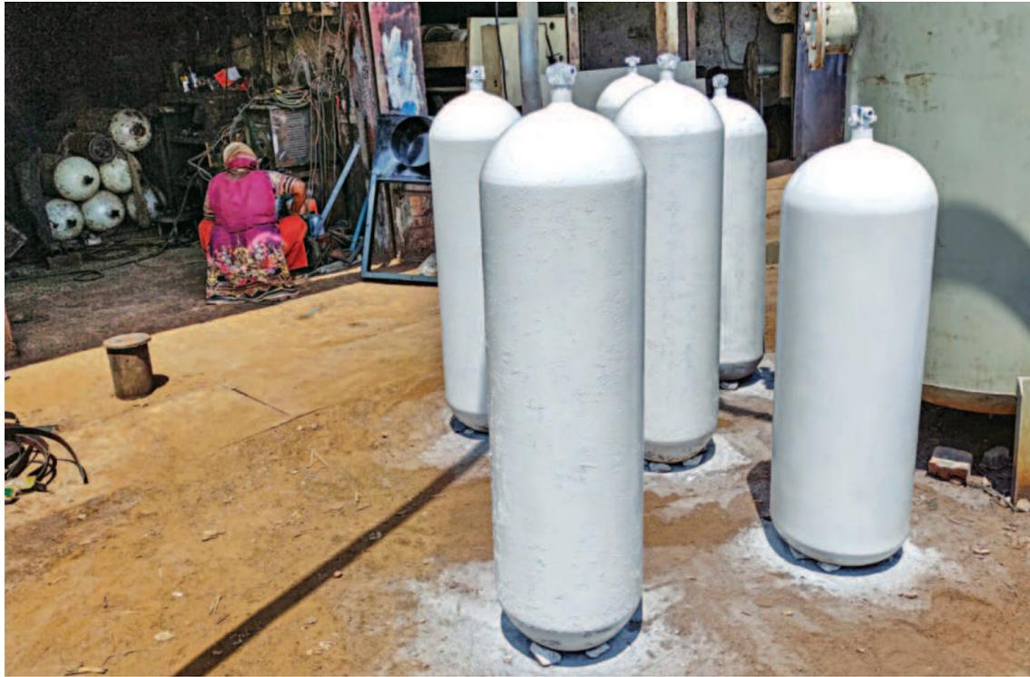
Old CNG cylinders being repainted for sale at a workshop on Mirpur's Mazar Road. The demand for such cylinders has increased as CNG conversion of vehicles picked up due to high prices of petrol and diesel, say the workshop workers. But old cylinders can be risky as they may not be fit for use. This photo was taken on Saturday.
