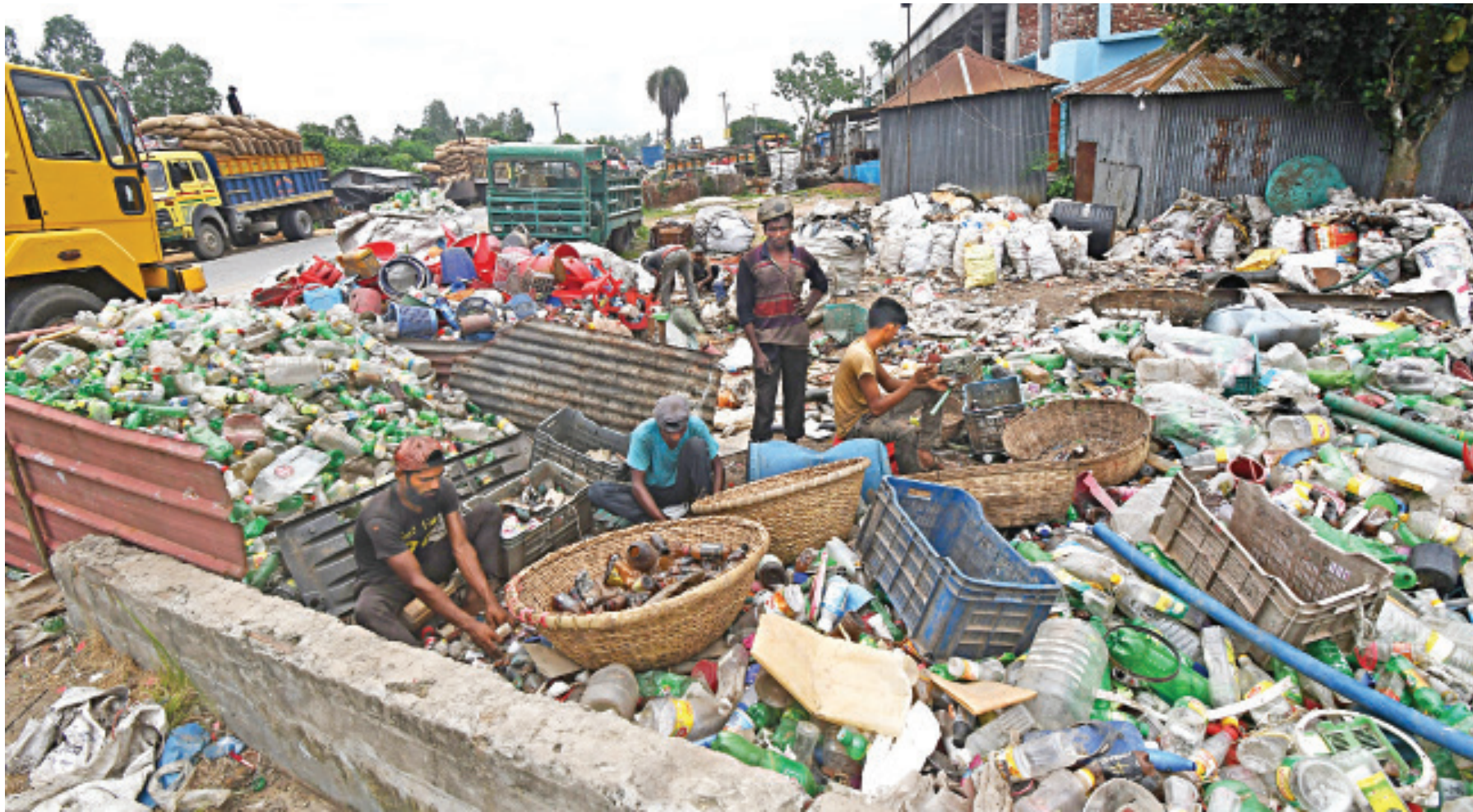
Discarded plastic materials collected by waste pickers being sorted based on colour and grade at a recycling facility by the Natore-Bogura regional highway in Jamtoli of Natore's Singra upazila. These will be shredded and washed prior to being turned into plastic pellets through a melting and compression process, and ready to be moulded into a new product. The photo was taken on Monday.
