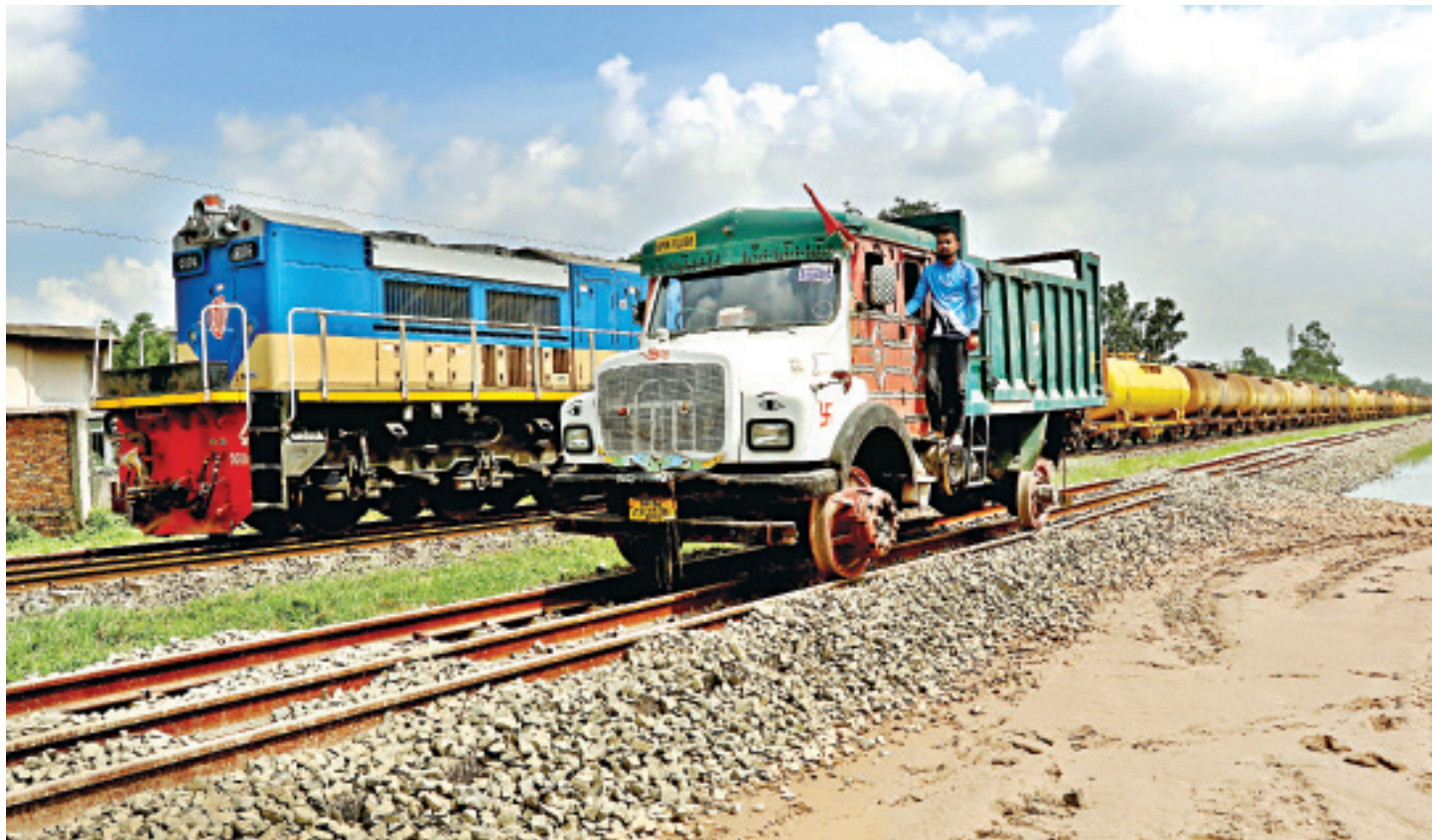
For many, it may appear unusual that a truck is rolling down a railway line carrying construction materials but conversions of such vehicles for building railway lines are quite common in the sector. The vehicle in question belongs to an Indian contractor building the Tongi-Joydevpur rail line in Gazipur.
