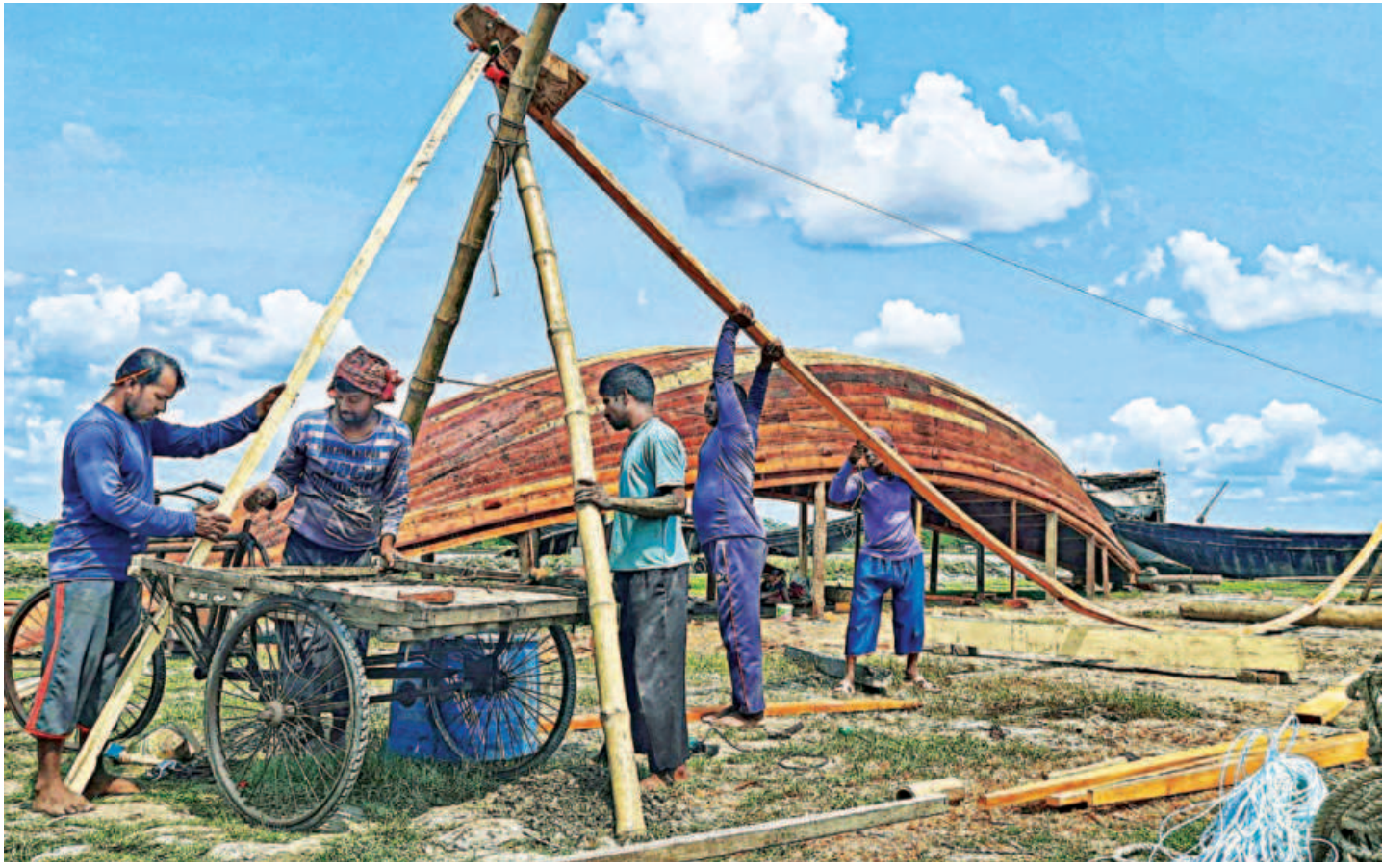
A trawler being built at Kulbaria Bazar of Khulna's Dumuria upazila. The vessel would be used for catching fish in the Bay of Bengal. Its manufacturing cost is around Tk 12 lakh, including the engine. It takes about one and a half months for five builders to finish the job. This photo was taken yesterday.
