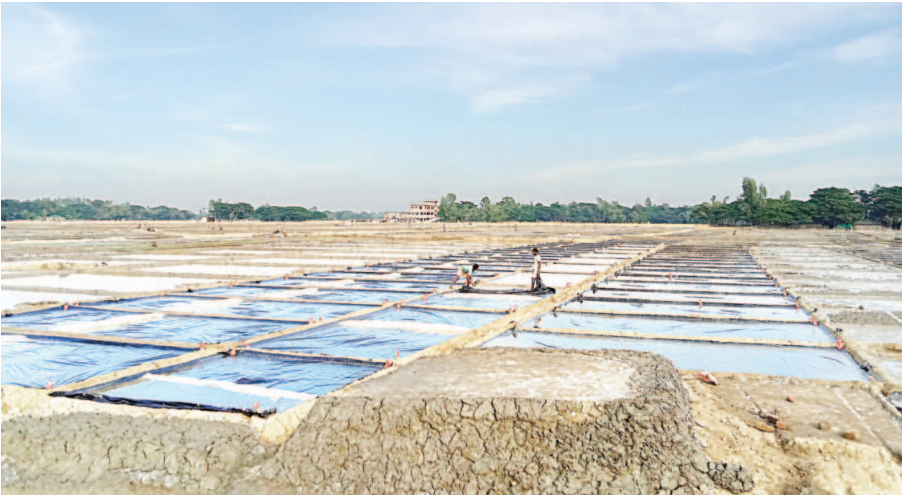
Saltwater left out to evaporate on plots of land in Durum area of Kutubdia upazila for the production of salt. Production mainly runs for five months from November to May in the coastal districts of Chattogram and Cox's Bazar. The photo was taken earlier this month.
