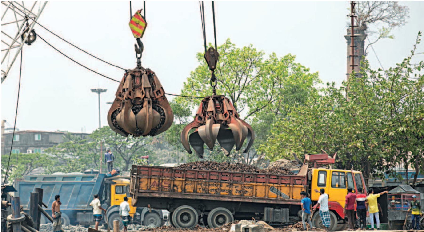
Imported scrap metal being unloaded from a ship and onto a truck in Majhirghat of Chattogram. Steel rods used in the construction industry are primarily made from scrap metal imported through the Chattogram port or metal collected from the breakdown of scrapped ships. The metal is melted to form billets which are later again melted to be poured into mould cavities to form rods of different shapes and sizes. The photo was taken recently.
