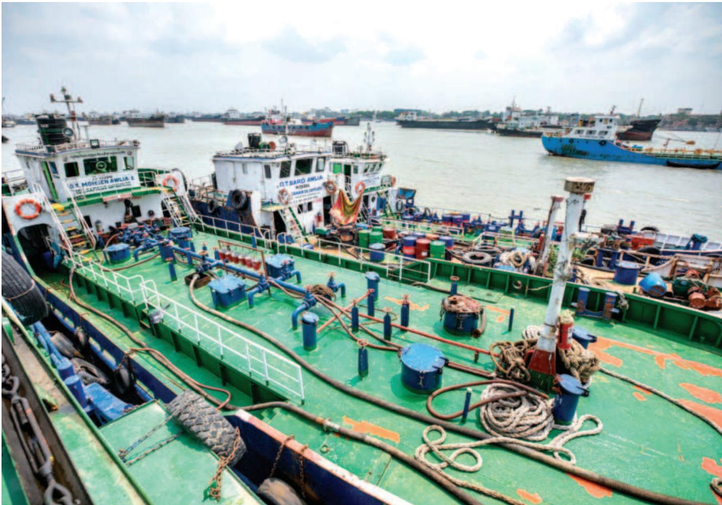
Replenishment tankers docked at Majhir Ghat in Chattogram yesterday. With tanks of 10 lakh to 11 lakh litre capacity, these vessels supply fuel to large ships further out at sea.
