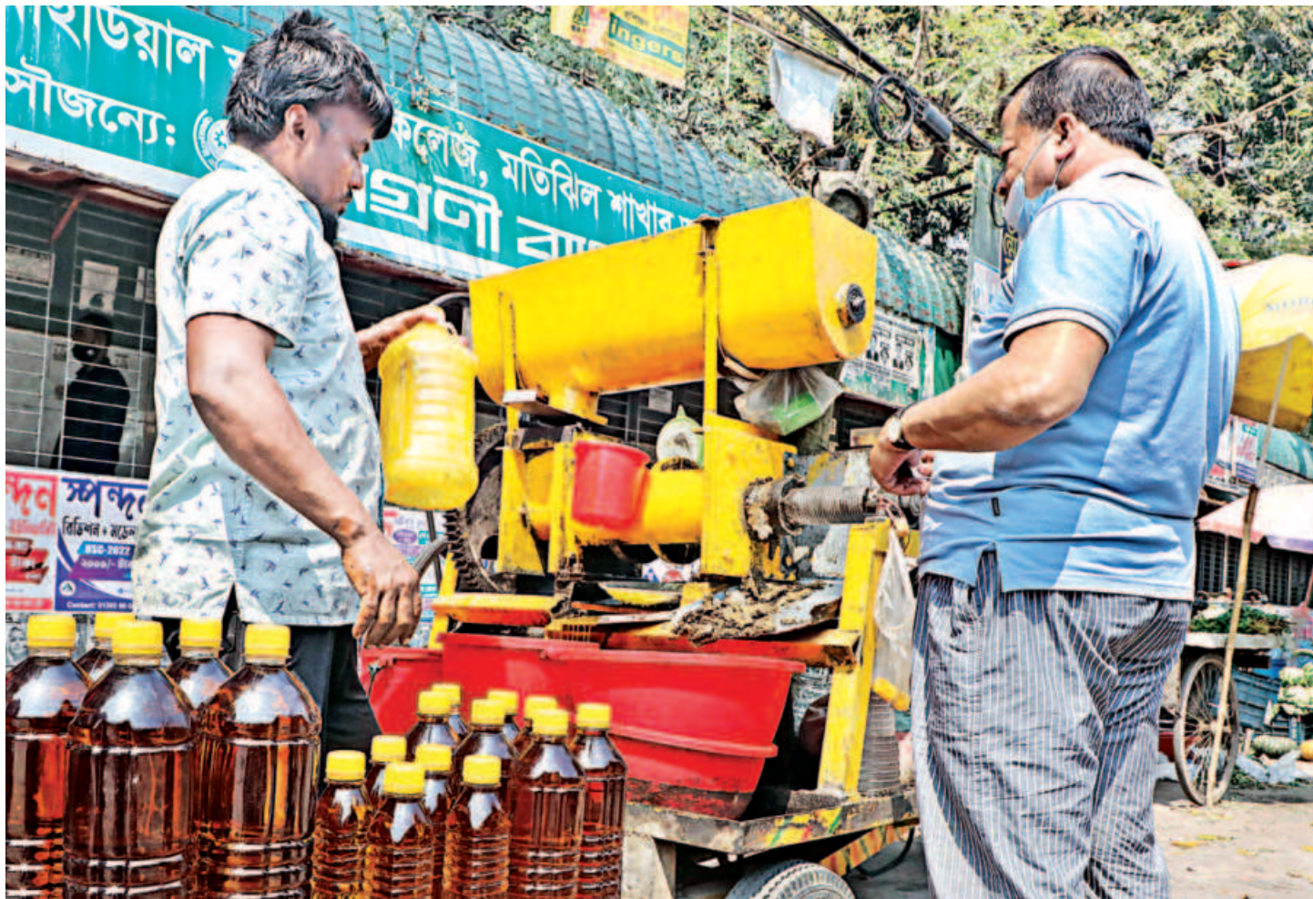
Mustard oil on sale for Tk 240 a litre in front of the Ideal School & College in the capital's Motijheel. The product is pressed out of seeds on a customised mini mobile mill comprising an expeller run by a diesel engine, all in full public view simply to give customers a sense of its purity. The photo was taken on Sunday.
