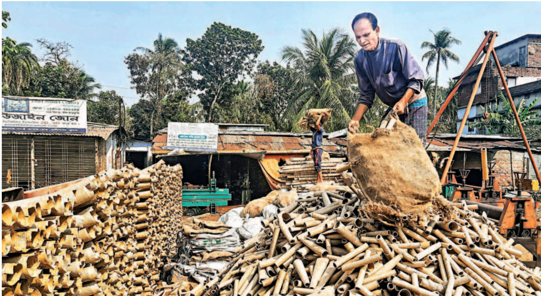
Spindles, also known as bobbins, made out of recycled paper being dried out in the sun. Jute mills purchase them for Tk 4 to Tk 8 per piece depending on the size to wind twine. This factory at Mujgunni Bus Stand in Khulna city has 16 workers who can manufacture nearly 60,000 spindles a month. The photo was taken on Saturday. PHOTO: HABIBUR RAHMAN
