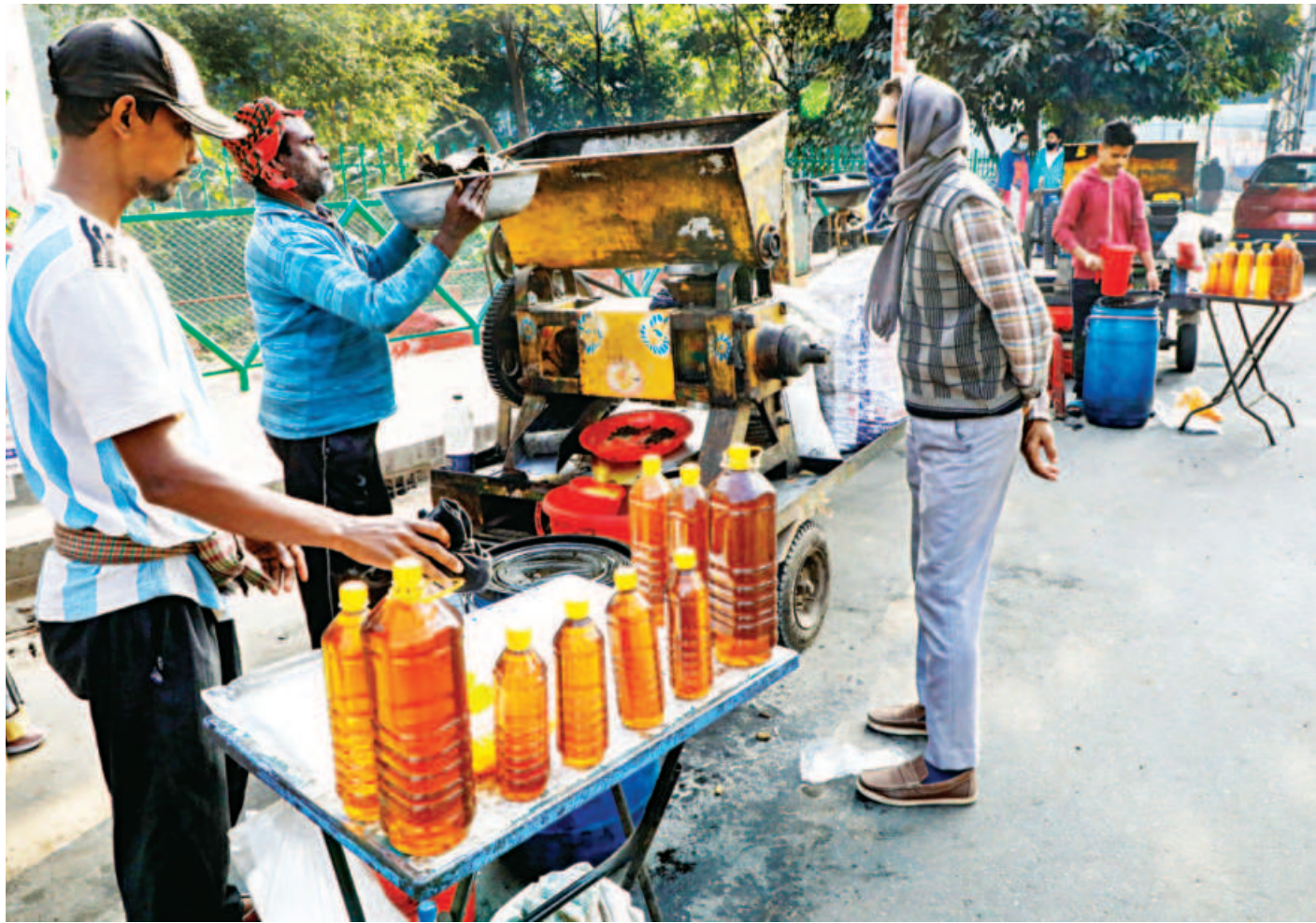
Two mobile expeller presses sell mustard oil for Tk 200 a kilogramme in the capital's Dhanmondi. Extracting the oil from seeds right before the eyes of customers assures of its purity, something most people are skeptical of in case of oil available in the markets. The photo was taken recently.
