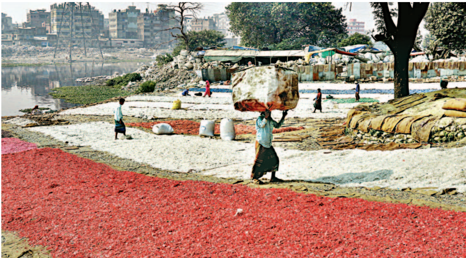
Scraps of red coloured plastic of the same type left out to dry in the sun at Kamrangirchar prior to being shipped off to be turned into recycled plastic pellets. Informal waste pickers collect discarded plastic for sale to traders, who then sort according to grade, shred and wash those for export. The polymers undergo a melting and compression process to be turned into recycled plastic pellets, ready to be moulded into a new product. The photo was taken recently.
