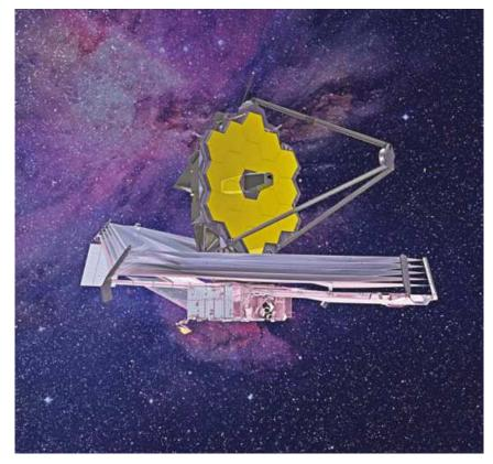
The telescope is unequalled in size and complexity. Its mirror measures 6.5 metres (21 feet) in diameter -- three times the size of the Hubble's mirror -- and is made of 18 hexagonal sections. It is so large that it had to be folded to fit into the rocket. That maneuver was laser-guided with NASA imposing strict isolation measures to limit any contact with the telescope's mirrors from particles or even human breath.
