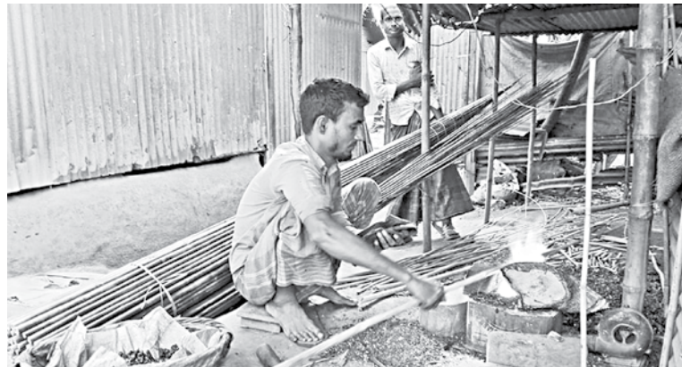
The process of making fishing rods includes cleaning and baking the bamboo sticks, supplied to the makers by local agents from Sunamganj.
