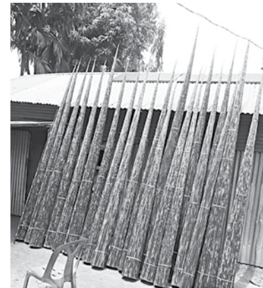
The process of making fishing rods includes cleaning and baking the bamboo sticks, supplied to the makers by local agents from Sunamganj.
