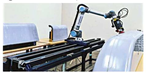
spraying on manufacturing lines. GrayMatter Robotics implements its software with commercially available robots, sensors and end-of-arm tools and enables them to treat any unique part. It uses machine vision and path planning to identify the part's geometry, pick up the right tool to process the part, figure out its material and which process to use, and then program the robot arm in the correct motion and execute the operation.
