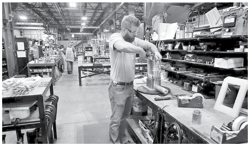
Sub-assembly worker Joel Dykema works on the sub-assembly of a transformer in the RoMan Manufacturing plant in Grand Rapids, Michigan, US.
