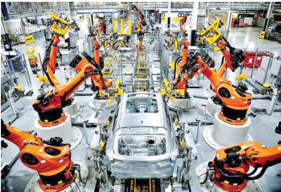
Autonomous robots assemble an X model SUV at the BMW manufacturing facility in Greer, South Carolina, US.
