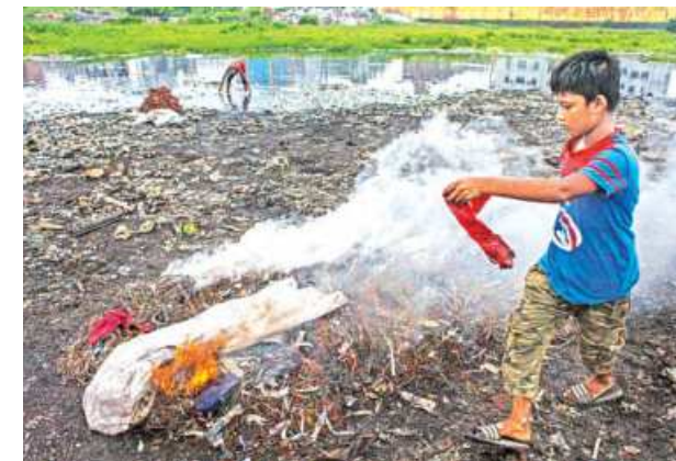
AT THE PRICE OF WHAT? Extracting copper from discarded electrical wires takes a couple of steps. The rubber of the outer layer is burned and the raw copper that's left is then washed and dried. At Dhaka's Kamrangirchar, a group of people bring sacks full of wires to this open area, burn them, and wash them in nearby water bodies. They get around Tk 300-350 for each kg of copper, but in the process end up doing a disproportionate amount of harm to the area's air and water. What's more, the workers don't even wear any protective gear to save themselves from the dark cloud of fumes they emit. These photos were taken recently.
