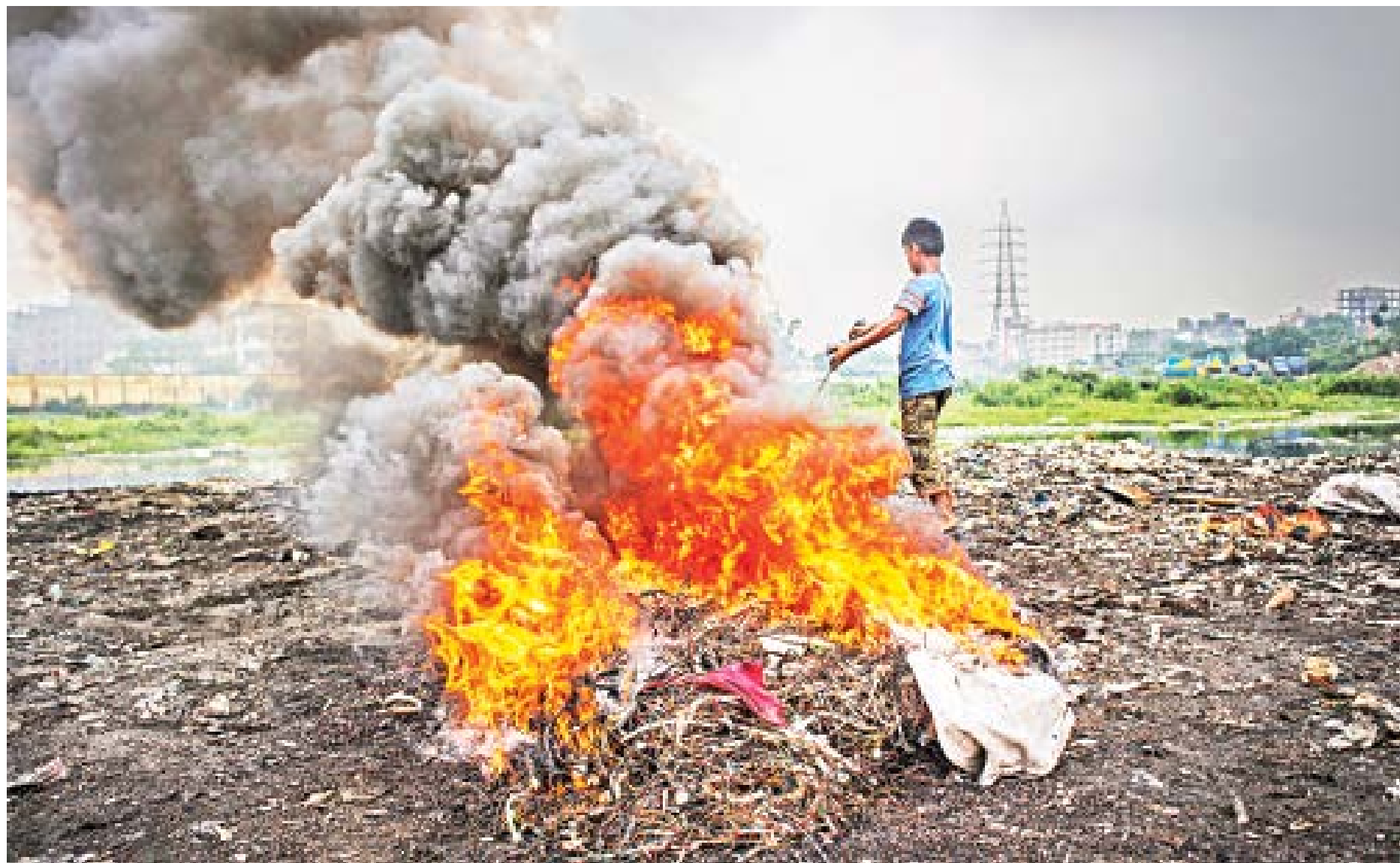
AT THE PRICE OF WHAT? Extracting copper from discarded electrical wires takes a couple of steps. The rubber of the outer layer is burned and the raw copper that's left is then washed and dried. At Dhaka's Kamrangirchar, a group of people bring sacks full of wires to this open area, burn them, and wash them in nearby water bodies. They get around Tk 300-350 for each kg of copper, but in the process end up doing a disproportionate amount of harm to the area's air and water. What's more, the workers don't even wear any protective gear to save themselves from the dark cloud of fumes they emit. These photos were taken recently.
