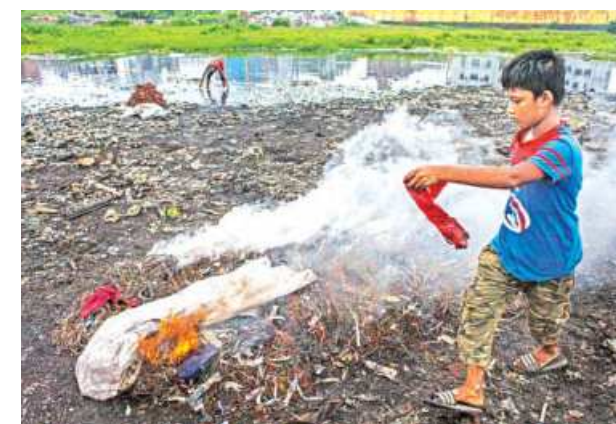
AT THE PRICE OF WHAT? Extracting copper from discarded electrical wires takes a couple of steps. The rubber of the outer layer is burned and the raw copper that's left is then washed and dried. At Dhaka's Kamrangirchar, a group of people bring sacks full of wires to this open area, burn them, and wash them in nearby water bodies. They get around Tk 300-350 for each kg of copper, but in the process end up doing a disproportionate amount of harm to the area's air and water. What's more, the workers don't even wear any protective gear to save themselves from the dark cloud of fumes they emit. These photos were taken recently.
