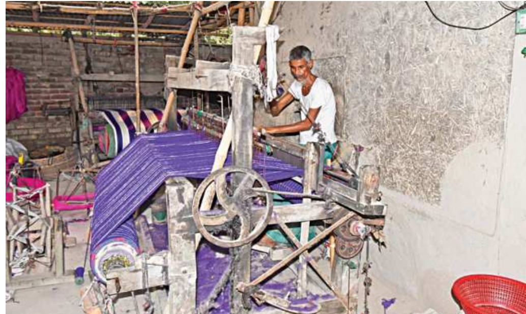
An elderly man is operating a handloom to make shawl based on yarn extracted from garment waste. Photo taken from SME cluster Bogura, Adamdighi.
