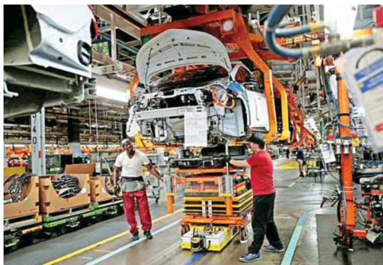
General Motors assembly workers connect a battery pack underneath a partially assembled 2018 Chevrolet Bolt EV vehicle on the assembly line at Orion Assembly in Lake Orion, Michigan, US on March 19, 2018.
