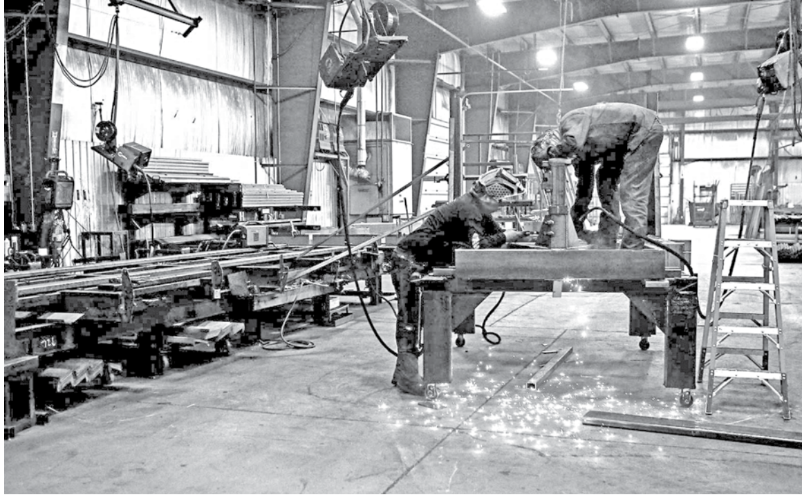
Workers weld an upper deck assembly at Look Trailers cargo trailer manufacturing facility in Indiana, US on April 1.
