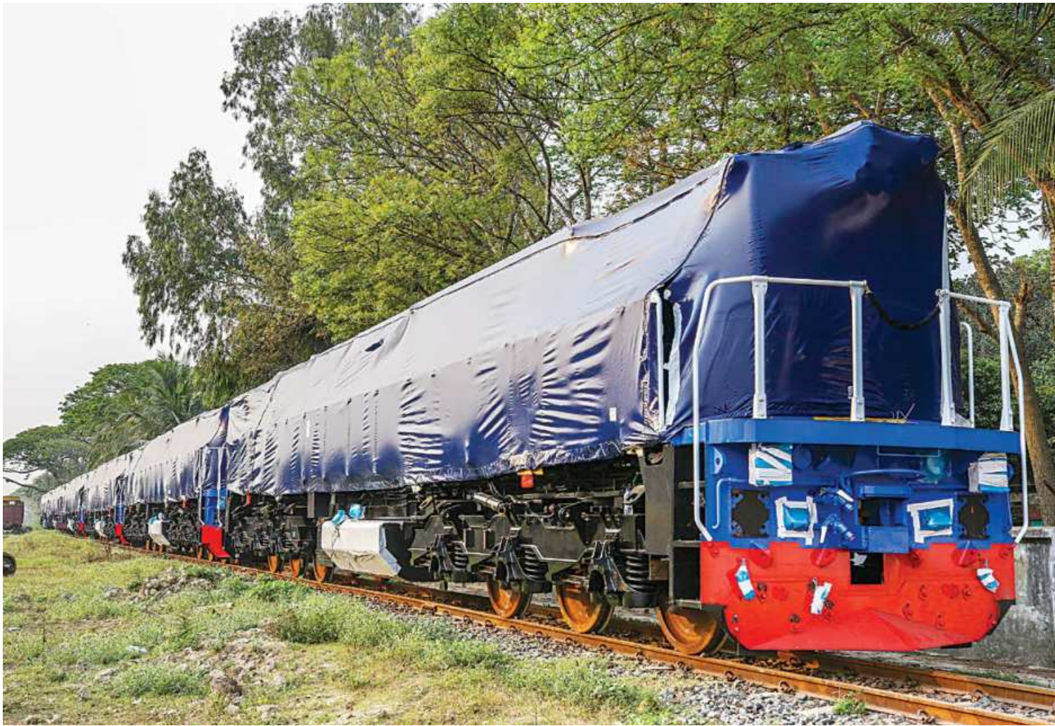
Eight of the 40 fast broad-gauge locomotives that Bangladesh Railway (BR) purchased from a company of the United States arrive in Chattogram. The locomotives have been given temporary metre-gauge undercarriages so that they could be taken to Dhaka’s Tongi Railway Station. From there, they will be sent to Parbatipur locomotive factory.
