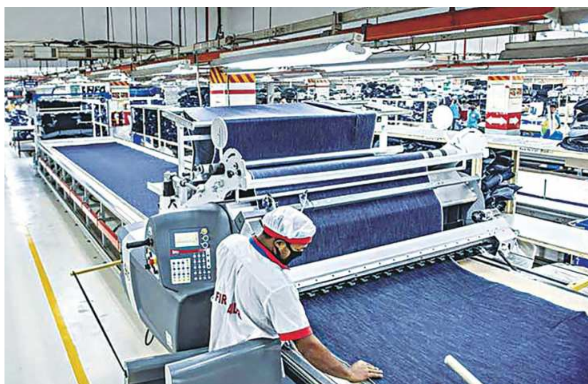
An automated spreading machine at Pacific Jeans.
