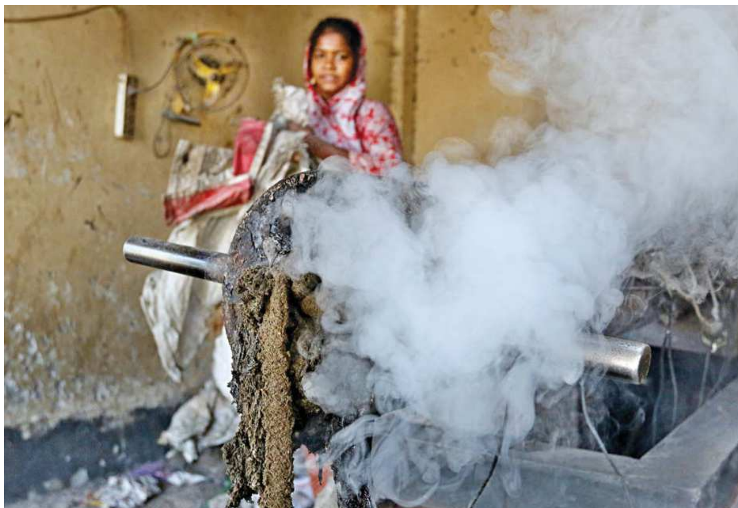
Ignoring health risks, a woman is melting plastic waste using an electric machine in the capital's Kamrangir Char area. At least a hundred factories in the area purchase waste plastic bottles from rag pickers, and melt and turn those into new plastic products. Meanwhile, the workers are not provided with any safety gear. The photo was taken recently.
