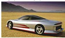
achieved with a 3.0 liter twin-turbo V6 making 350 HP delivering power to all four wheels, with a 0-100 of just under five seconds. Much like all other concept cars on this list, the car was far too advanced for mass production. However technologies derived from this car did make it to production models, such as the Mitsubishi GTO.
