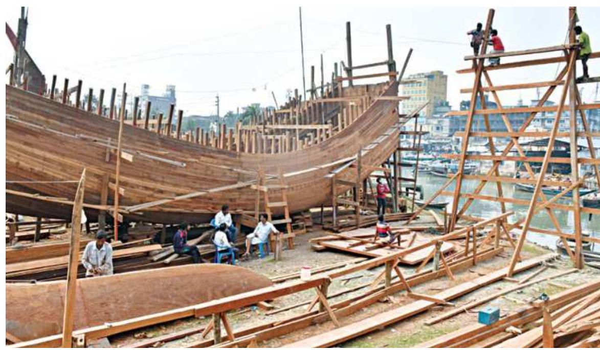
Trawlers, used for catching fish in the sea, is being made in Rasulpur area of Barisal City. Each of these boats could be as high as 50 feet and it takes months to build one. The photo was taken a couple of days ago.
