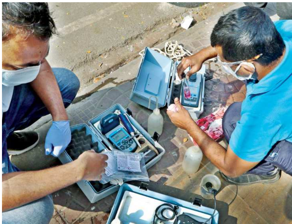
Wasa personnel test the quality of water being distributed throughout Dhaka city at Palashi area, after collecting samples from the supply line. However, one cannot help but wonder whether conducting such a test out on the streetside is really the best approach. The photo was taken yesterday.
