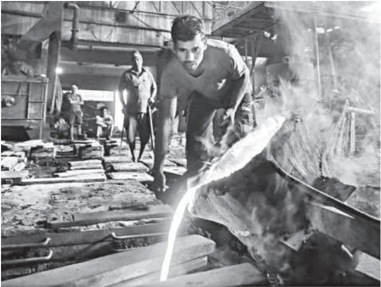
A worker pours molten iron from a ladle to make automobile spare parts inside an iron casting factory in Ahmedabad, India.
