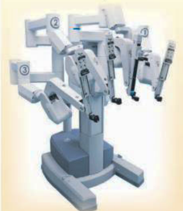
The robotic system's arms, fitted with tiny instruments, are inserted through small incisions into the surgical site.
