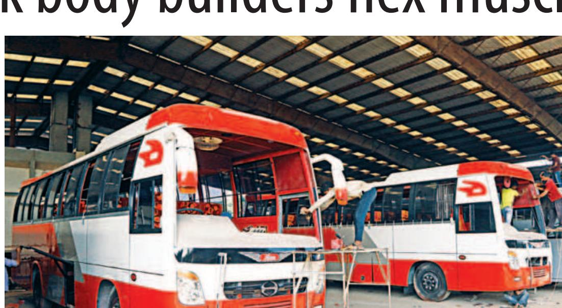
Bus bodies being manufactured at a workshop of Aftab Automobiles in Gabtoli, Dhaka. Inset, two men put together foam and covers on seats.
