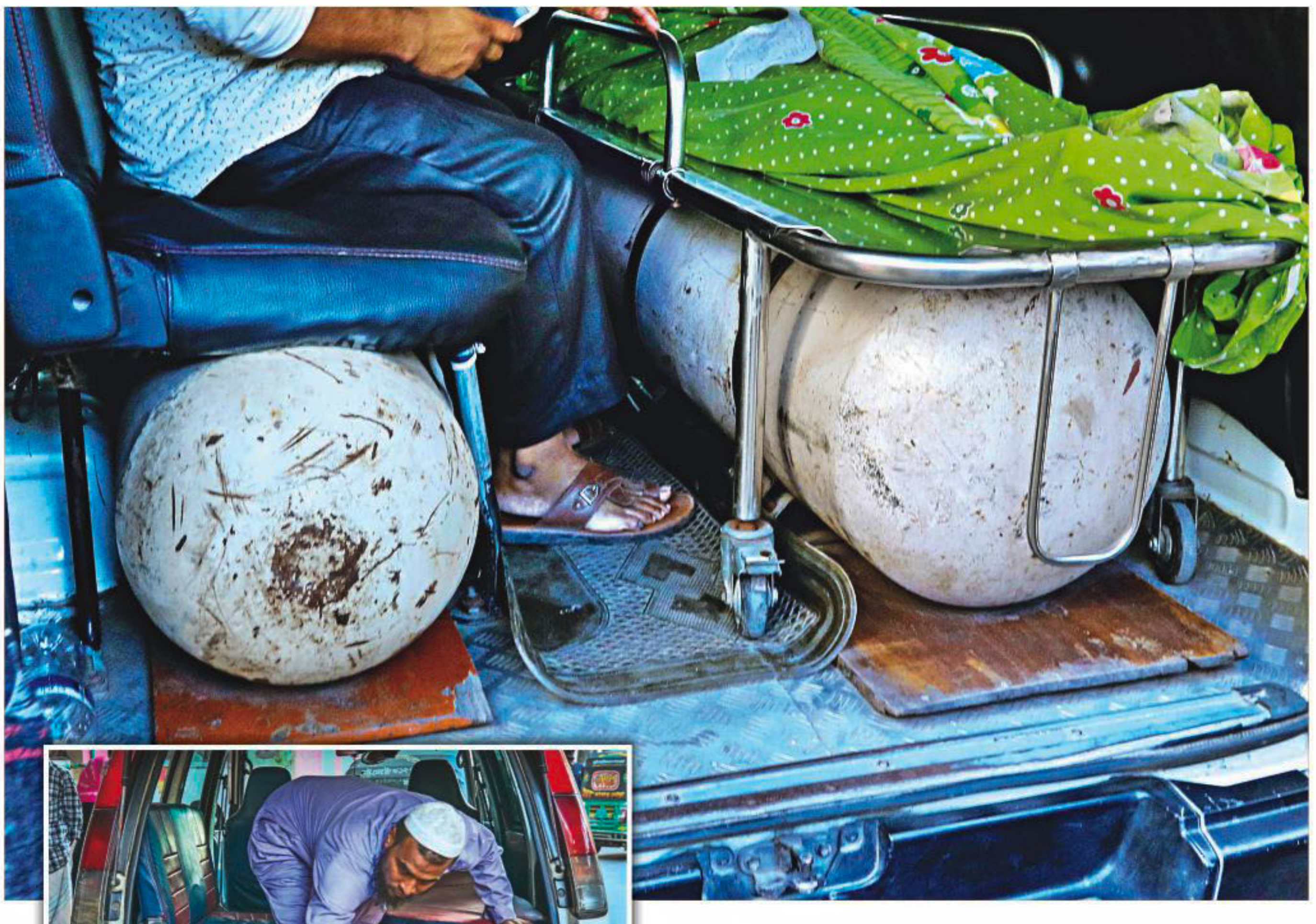
Gas cylinders are installed under the stretchers and benches in ambulances. CNG cylinders have caused fatal accidents in the past. Only two days ago, three people died when a cylinder inside an ambulance exploded in Chattogram's Anwara apazila. The photos were taken at the Dhaka and Chattogram medical college hospitals yesterday. PHOTO: ANISUR RAHMAN, RAJIB RATHAN
